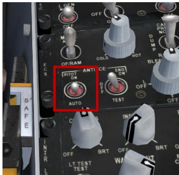
Figure 2 PITOT HEAT SWITCH (Activates Takeoff Trim)
