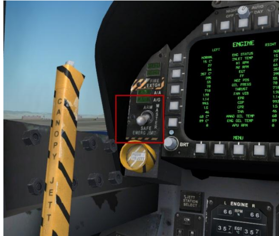
Figure 1 MASTER ARM SWITCH (deactivates FCS)
